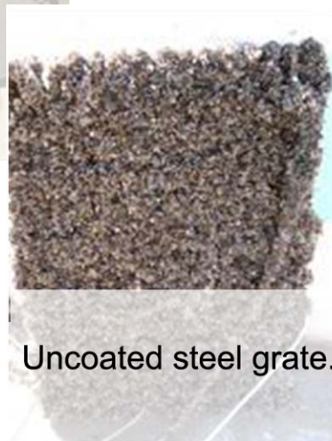
Flame sprayed zinc metalizing contrast between plates (minimal flowing conditions) and grates (flowing conditions).
