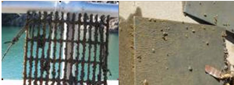
Flame sprayed zinc metalizing contrast between plates (minimal flowing conditions) and grates (flowing conditions).
