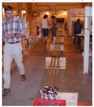
Very high zebra mussel kill (>95%) was consistently achieved in 6-hr treatments at 100 ppm inside a NYPA hydropower plant under flow-through conditions (3 replicate pipes 17 m in length were used in this trial). Experiments to date indicate that there should be no limit on the length of pipe that can be successfully treated.
