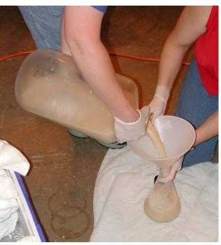
Pouring suspension of bacterial cells in preparation for pipe treatments within power plants. Advances in fermentation have allowed increasingly larger volumes of bacteria to be produced, thus allowing larger volumes of water to be treated in pipes.
